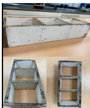
Figure 1 - Improved molder for multi-nutrient lick block production
